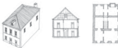
6. CASA DE ESCADA CENTRAL CENTRAL STAIRCASE HOUSE
